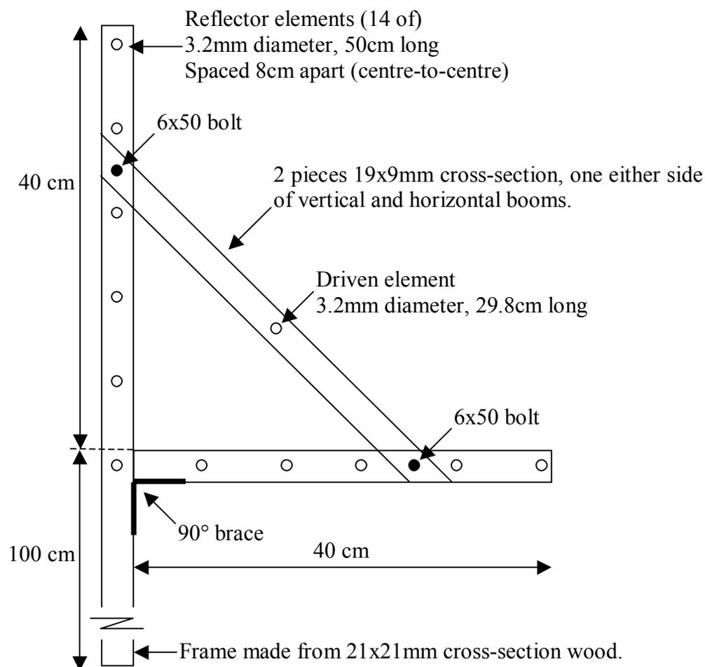
**Figure 2 – Construction Details**
