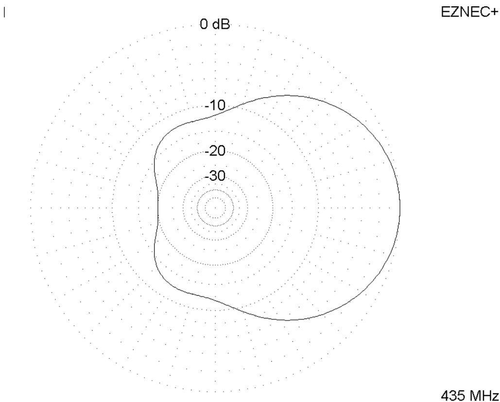
Figure 4 – Azimuth pattern at 30 degrees elevation
