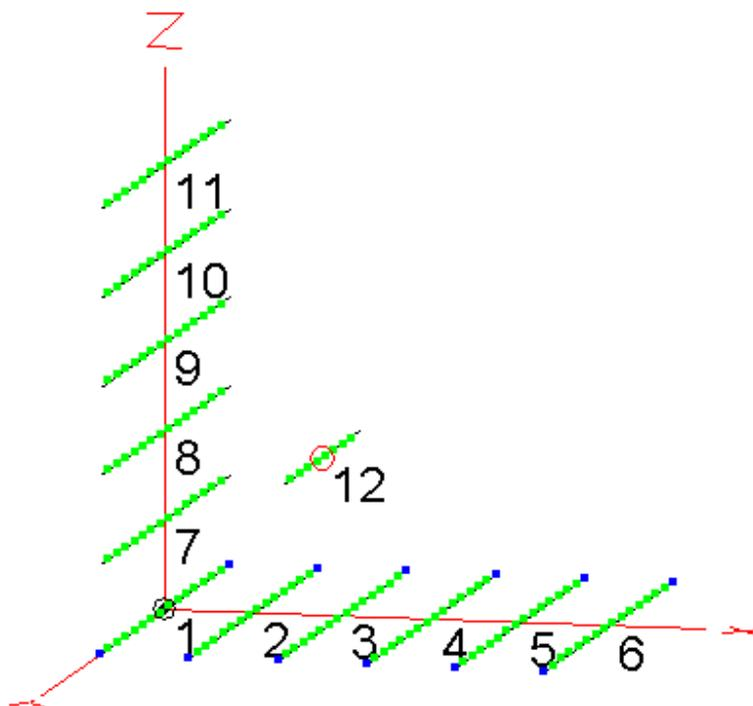
Figure 1 – Layout of the Corner Reflector
