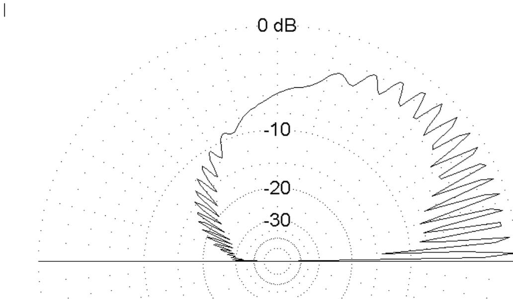
Figure 3 – Elevation pattern at 435MHz mounted 5m above ground.
