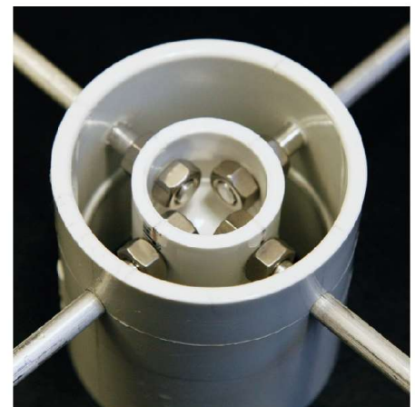
Figure 2 — The completed feed-point assembly.
