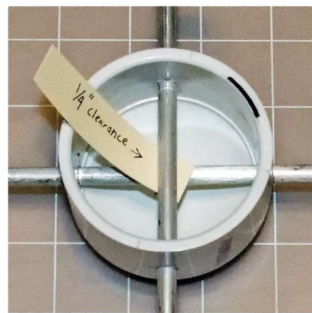
Figure 4 — The rods at 90° orientation are displaced so there is a \frac{1}{4} -inch gap between them.
